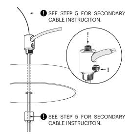
**4** Weave power cord from LIGHT ENGINE through all necessary parts based on lamp model.
