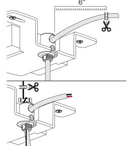
Pull SECONDARY CABLE down through STRAIN RELIEF A until it stops.
