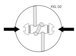
The location of STRAIN RELIEF B will determine the lamp's hang height.
