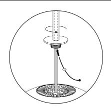
Feed Steel cable (included) through the POST until the crimped ball end bottoms out. **2** Peel protective later from VHB tape (included) and secure DRIVER to MOUNT BRACKET.
