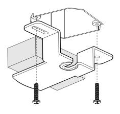
7 Unthread both set screws using included hex tool. Weave cables(s) through CANOPY NUT, CANOPY, AND STRAIN RELIEF.
