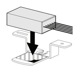
Thread POST onto LIGHT ENGINE. (NOTE! For Bola Disc; DISC will be trapped in between POST and LIGHT ENGINE. See FIG. 01).
