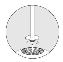
**3** Secure MOUNT BRACKET to junction box using appropriate anchoring hardware (included).
