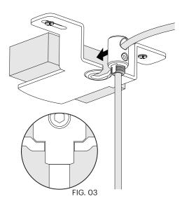
If employing SECONDARY CABLE, add included STRAIN RELIEF B now. Feed cable through both holes and tighten screws as demonstrated in Figure 02.
